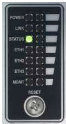
Figure 5. Location of Reset Switch
