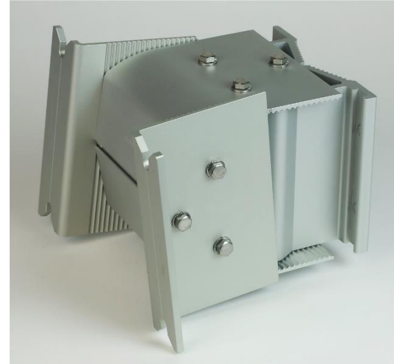
Figure 5: Twisted Bracket Ears
