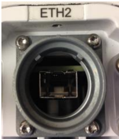
Figure 5 : Device Side Radiall OSIS Push-Pull SFP Connector
