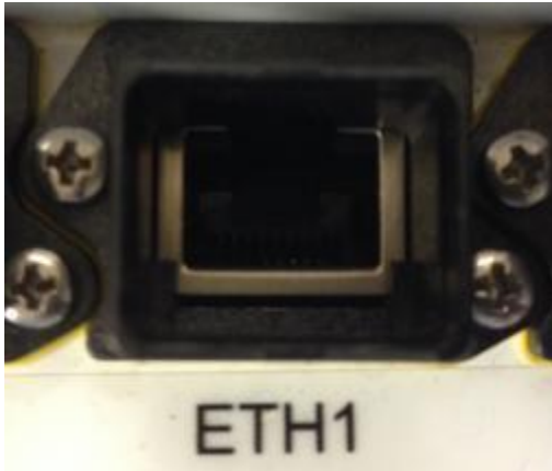
Figure 2: Device Side Harting Push-Pull RJ-45 Connector
