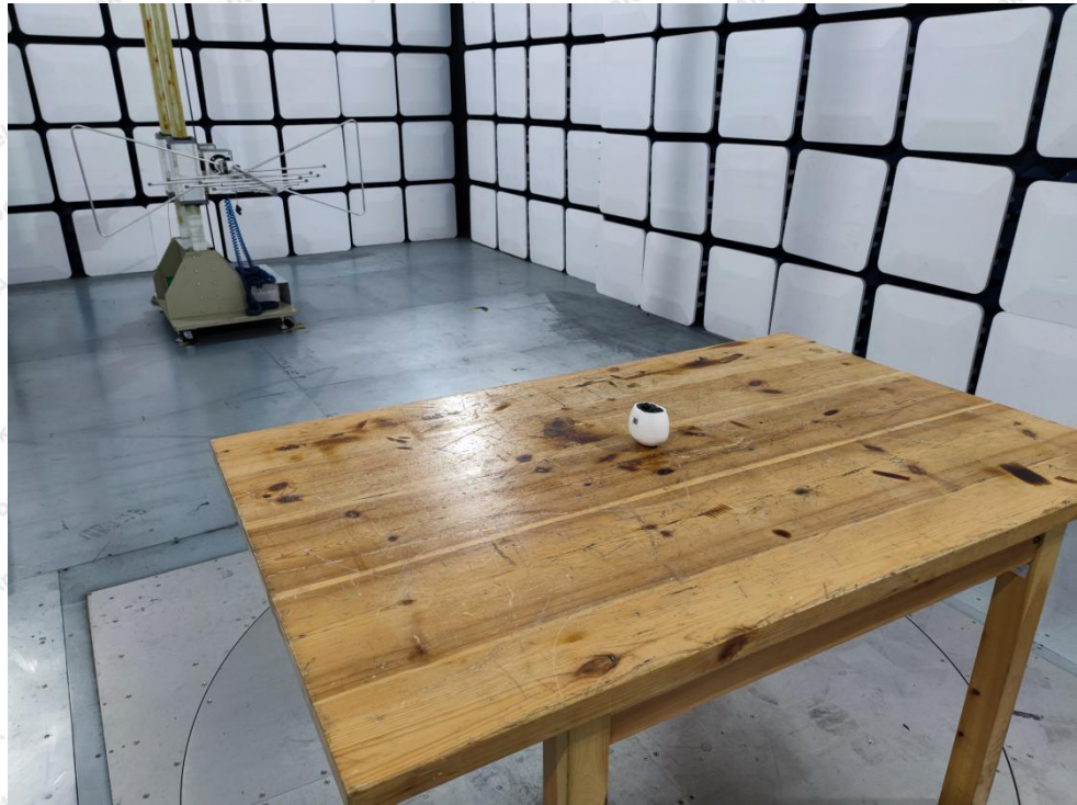
Photo of Radiation Emission Test
