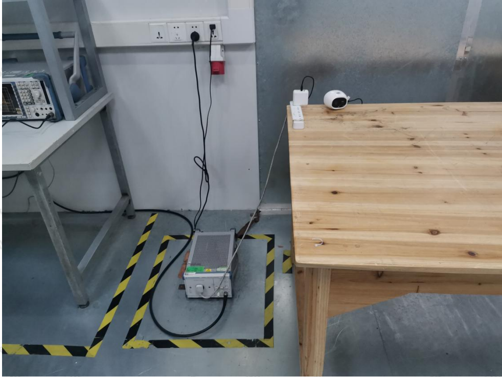
Photo of Power Line Conducted Emission Test
