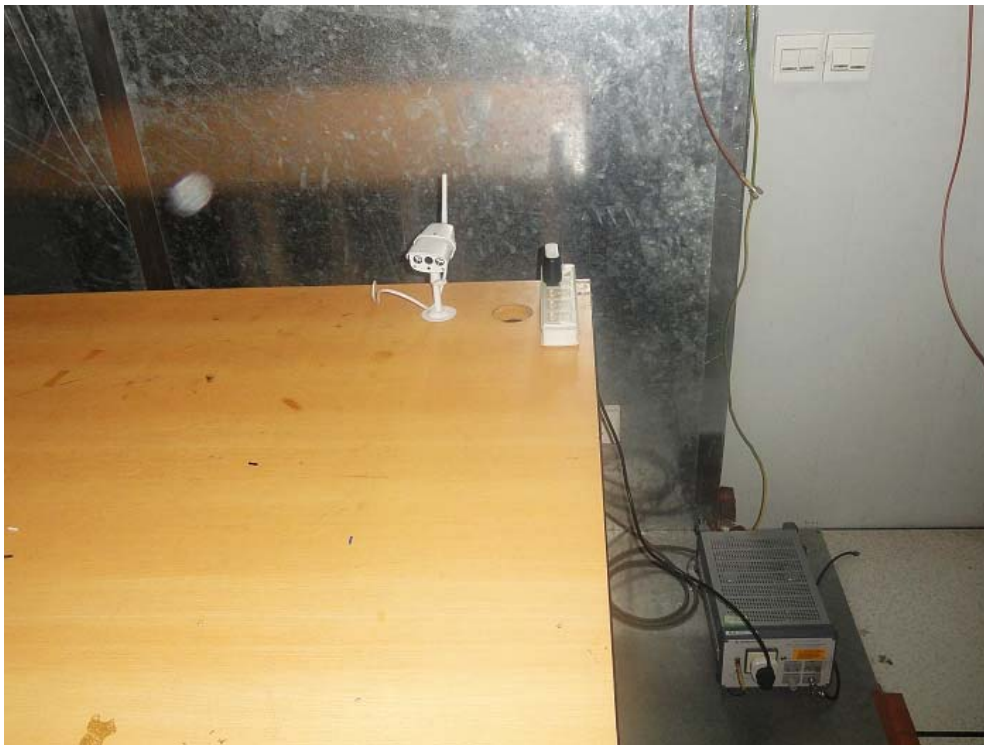
Conducted Emission Test Setup:
