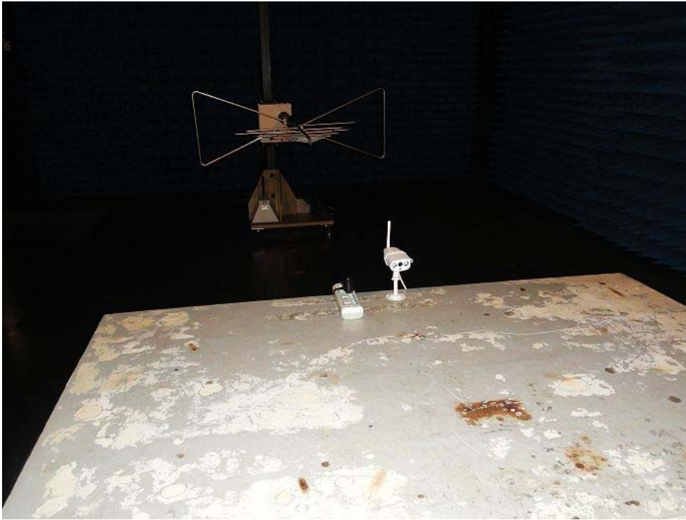
Radiated Emission Test Setup:
