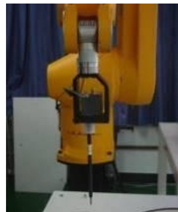
Picture C.3 E-field Probe
