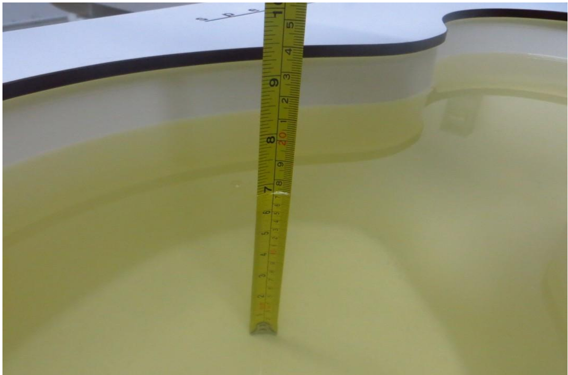
Picture 7-1: Liquid depth in the Head Phantom (835 MHz) (depth=15.6cm)
