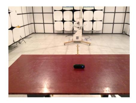
**15C Radiated Emission Test Setup**
