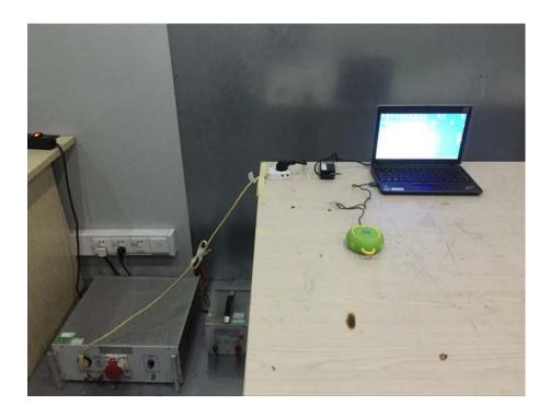
Radiation Emission Test Setup (Below 30MHz)
