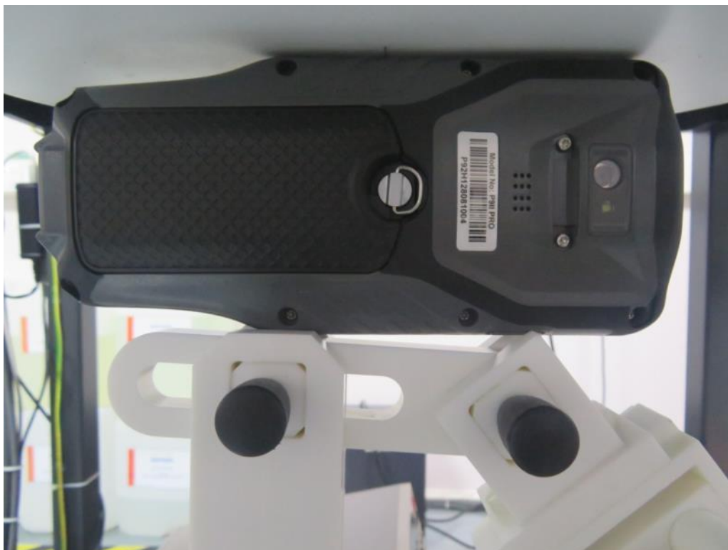
0mm body-worn Right Side Setup Photo (hotspot)
