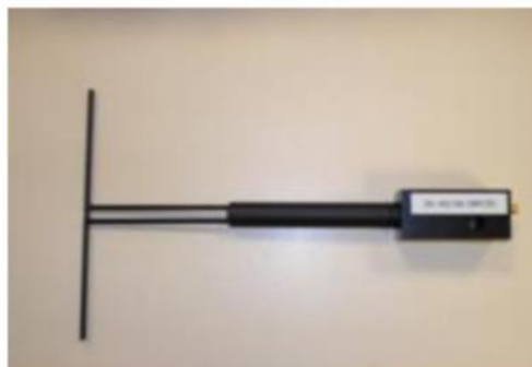
Figure 1 – Satimo COMOSAR Validation Dipole
