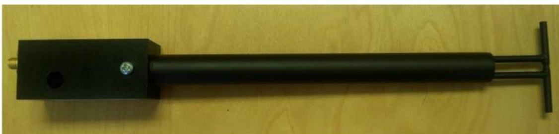
Figure 1 – MVG COMOSAR Validation Dipole
