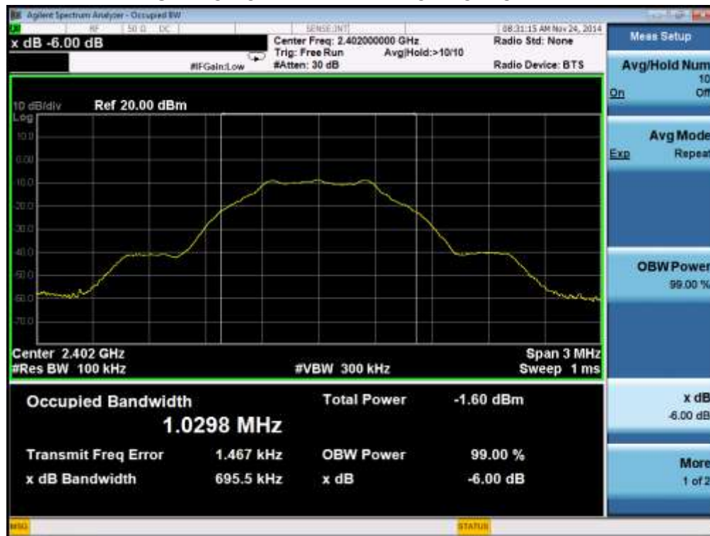
TEST PLOT OF BANDWIDTH FOR LOW CHANNEL
