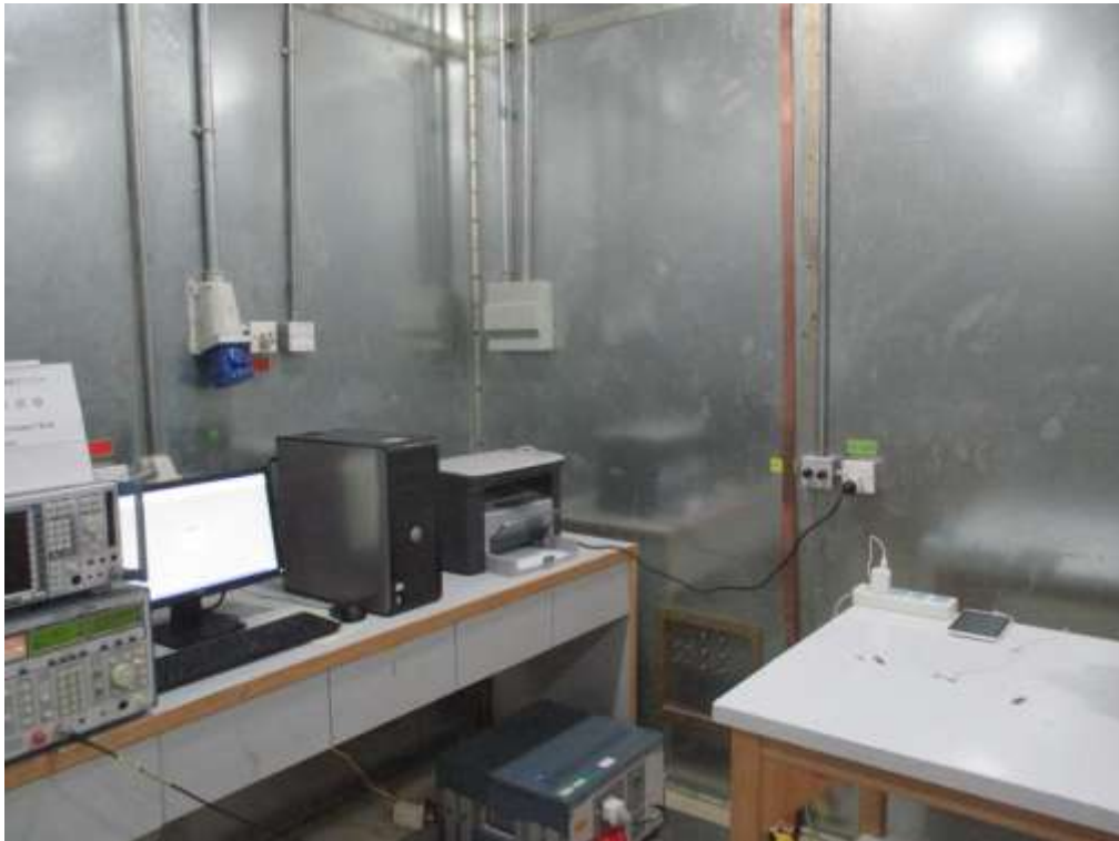
FCC RADIATED EMISSION TEST SETUP
