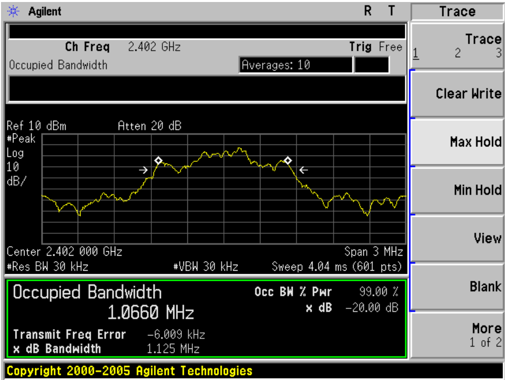
TEST PLOT OF BANDWIDTH FOR LOW CHANNEL
