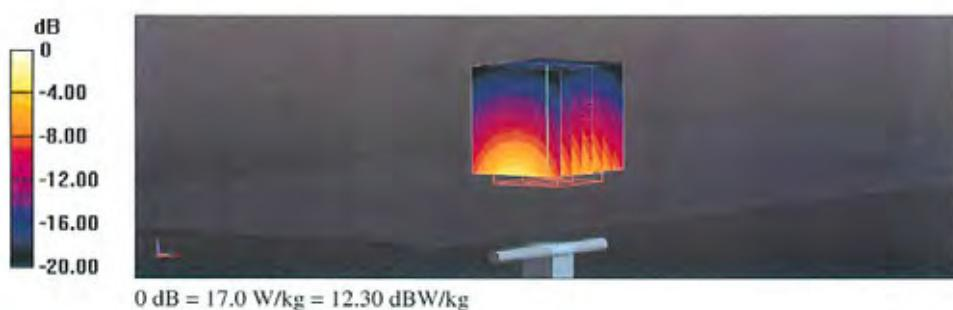
**Impedance Measurement Plot for Body TSL**
