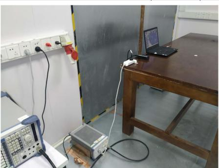
Conducted Emissions at AC Power Line (150kHz-30MHz)
