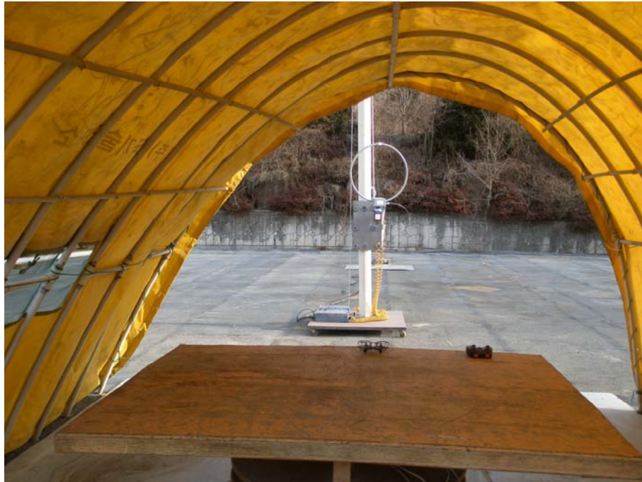
Photograph 1 : Setup for radiated Emissions (above 30 MHz)
