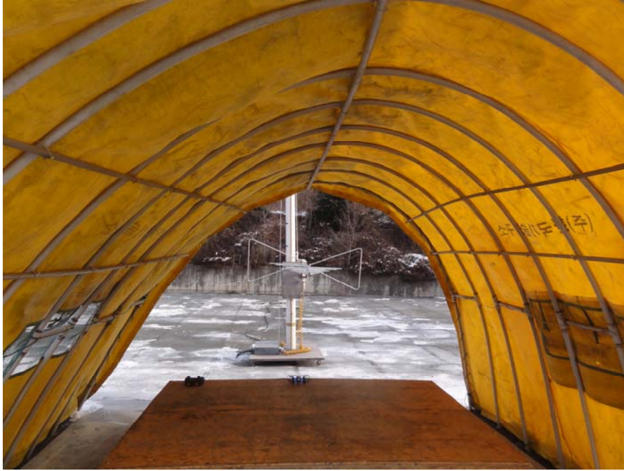
Photograph 2 : Setup for radiated Emissions (above 1 GHz)
