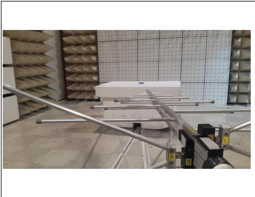
**B. Photo of Radiated Spurious Emission Test (Above 1 GHz)**
