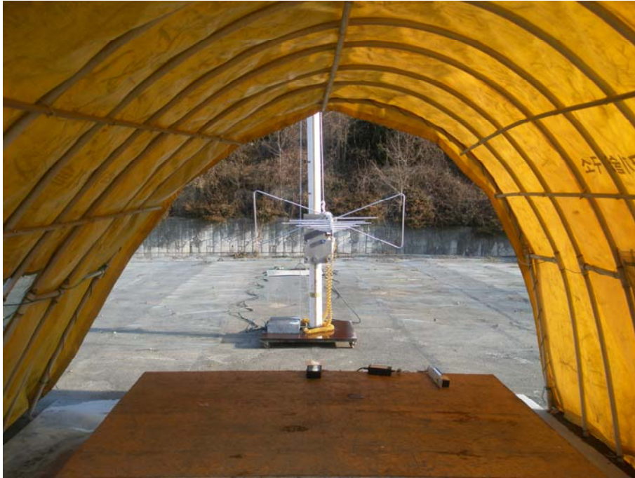
Photograph 2 : Setup for radiated Emissions (above 30 MHz)
