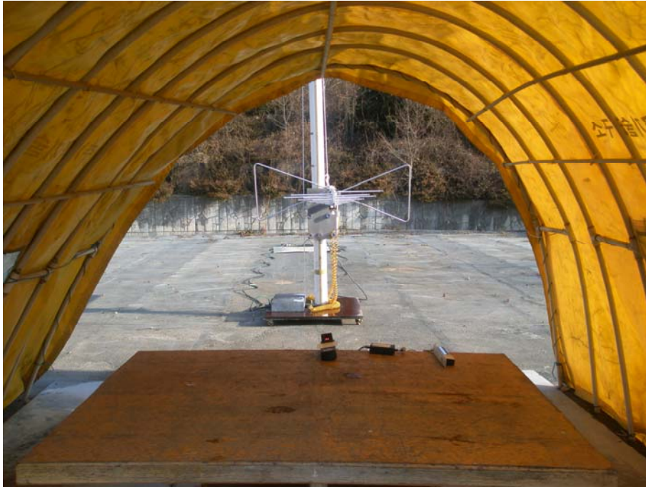
Photograph 2 : Setup for radiated Emissions (above 30 MHz)
