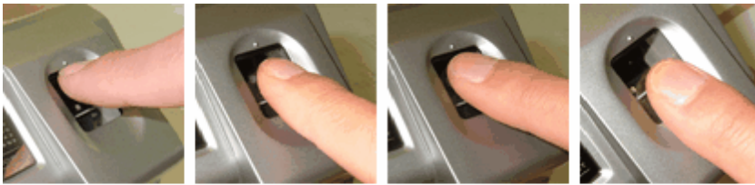
Figure 1: Improper Alignment Causes Problems
