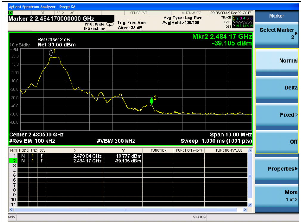
(Channel = 78, Band edge, GFSK Mode)
