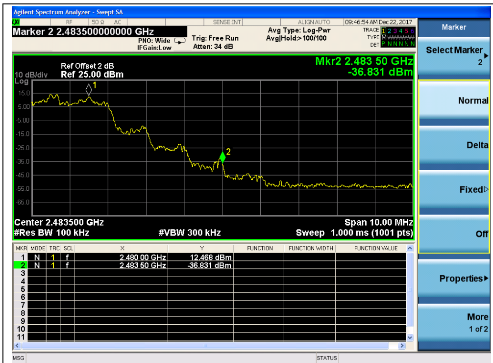
(Channel = 78, Band edge with hopping on, 8-DPSK)
