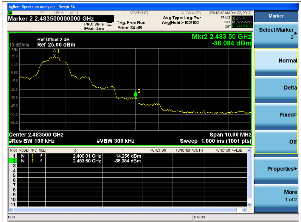
(Channel = 78, Band edge, \pi/4 -DQPSK)
