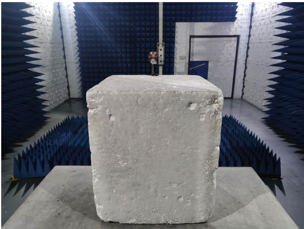
RADIATED EMISSION TEST SETUP ABOVE 1GHz
