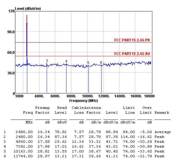
Test mode: 2480MHz **Polarization: HORIZONTAL**
