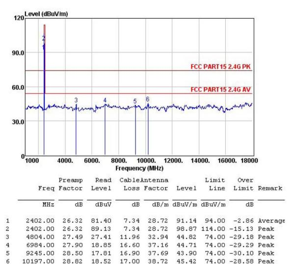
Test mode: 2402MHz Polarization: HORIZONTAL
