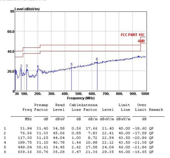
Test mode: 2402MHz Polarization: VERTICAL
