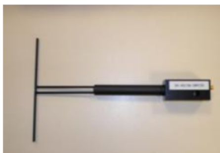
Figure 1 – Satimo COMOSAR Validation Dipole
