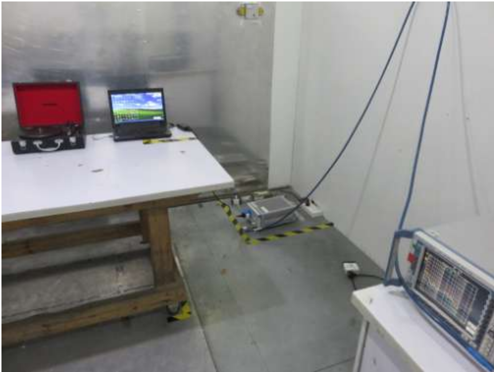
FCC RADIATED EMISSION TEST SETUP
