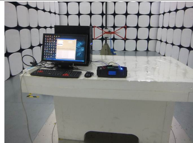
Radiated Spurious Emissions Test Setup Below 1GHz
