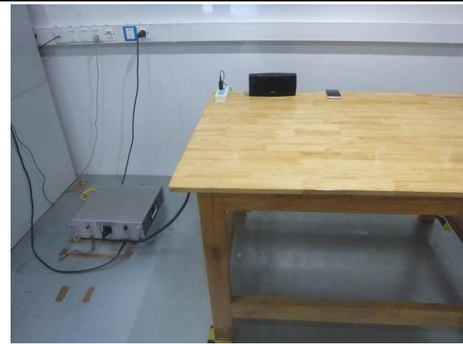
Conducted Emissions Test Setup Front View
