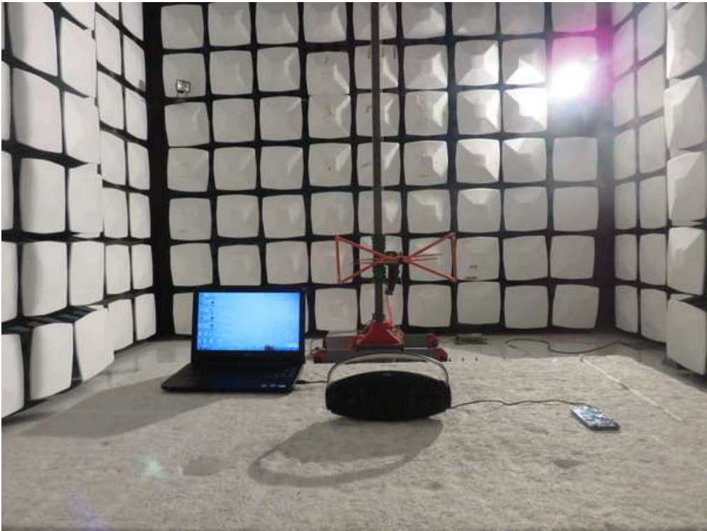
FCC RADIATED EMISSION TEST SETUP
