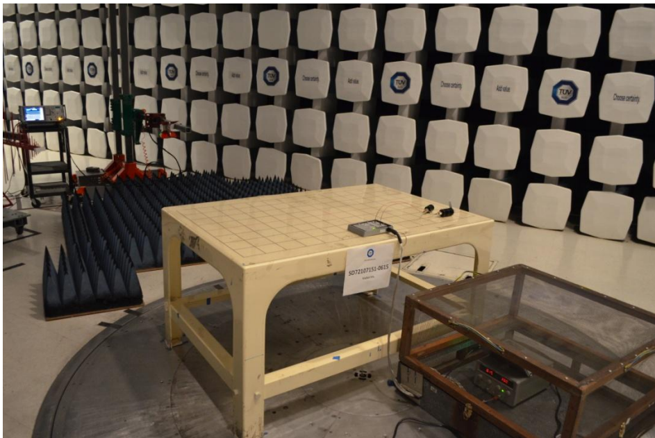
Setup for Satellite test Radiated Emission Above 1GHz Front and Back
