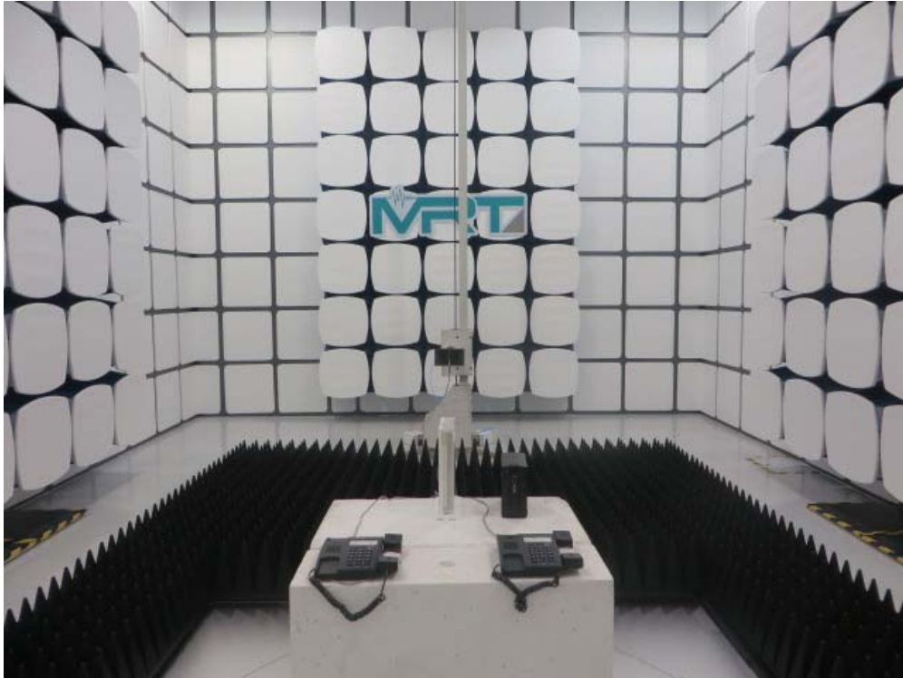
Description: Front view of Radiated Emission Test Setup for 1 ~ 18GHz (854G-2)
