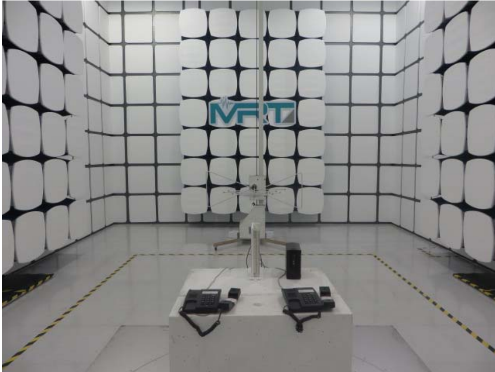
Description: Front view of Radiated Emission Test Setup for 30 ~ 1000MHz (854G-2)
