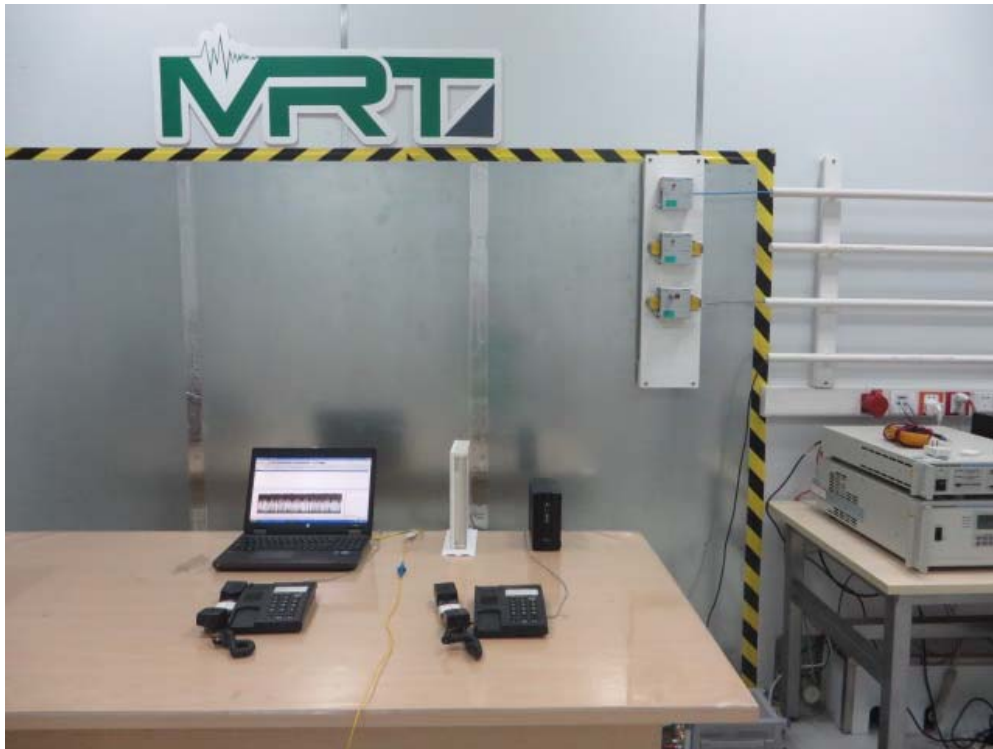
Description: Back view of Conducted Emission Test Setup (854G-2)
