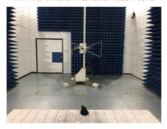
RADIATED EMISSION TEST SETUP ABOVE 1GHZ
