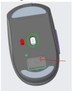
2: Turn ON the power switch to the ON position (up and down, and OFF in the middle), and click the left or right mouse button arbitrarily in the blank space of the computer desktop. When you move the mouse, the cursor can move. You can easily use your 2.4G wireless optical mouse at this time.
