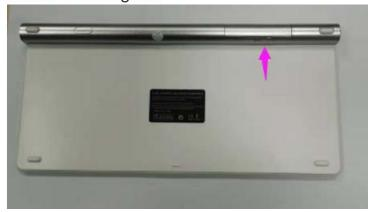
2: Put 2 3A batteries into the collection box of the keyboard
