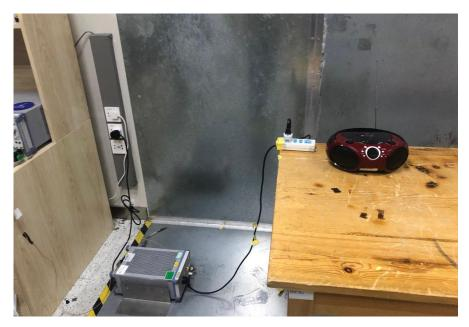
Radiated Emissions From 30MHz-1000MHz
