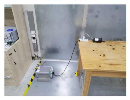
Radiated Emissions From 30MHz-1000MHz
