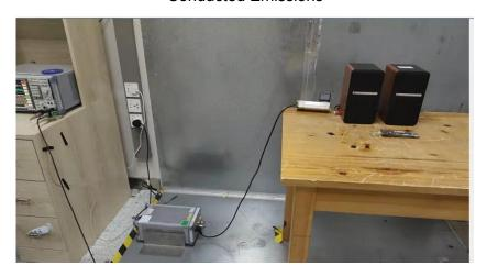
Radiated Emissions From 30MHz-1000MHz
