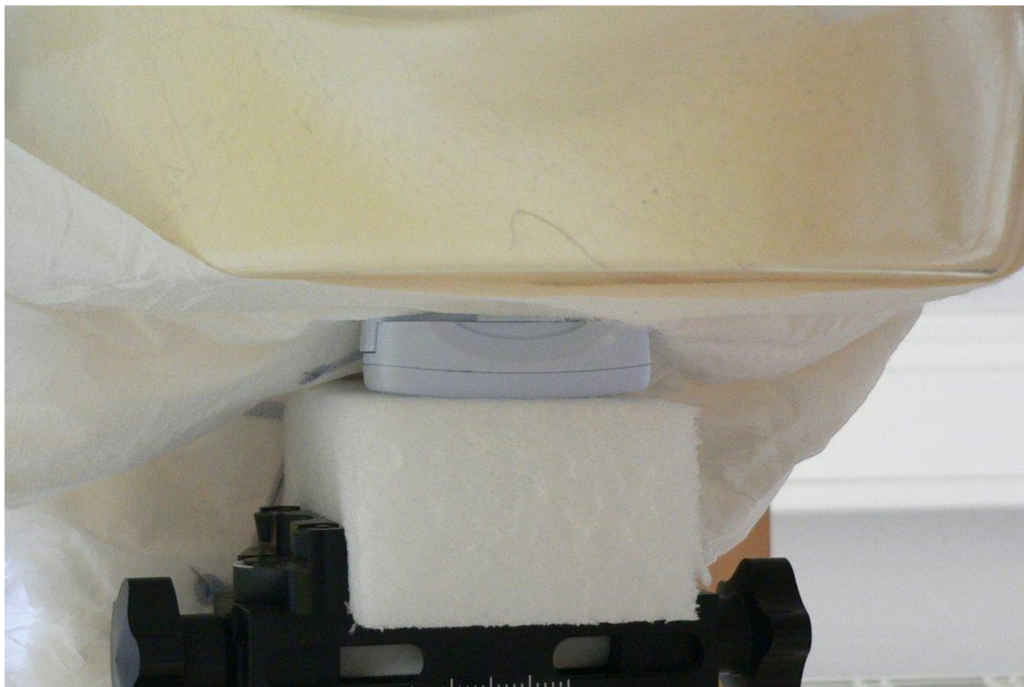
Fig. 9: Position 1, use case scenario, TENA Identifi Logger from SCA Hygiene Products in combination with a diaper below the flat part of the SAM phantom.
