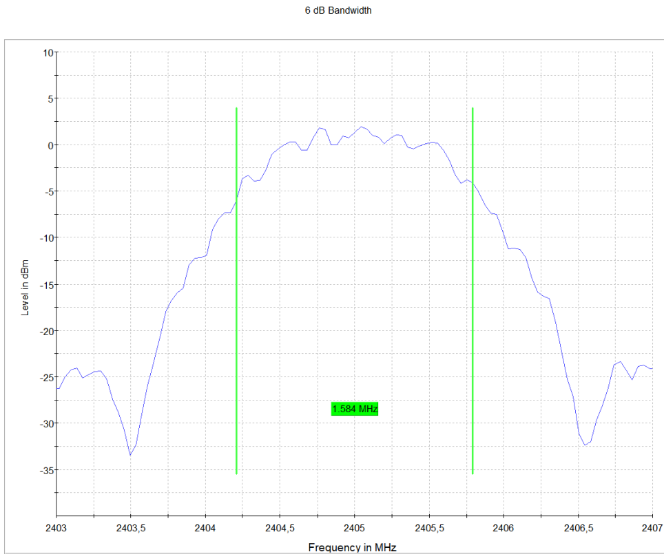
Screenshot: Occupied 6 dB bandwidth Measurement. low channel. 802.15.4.
