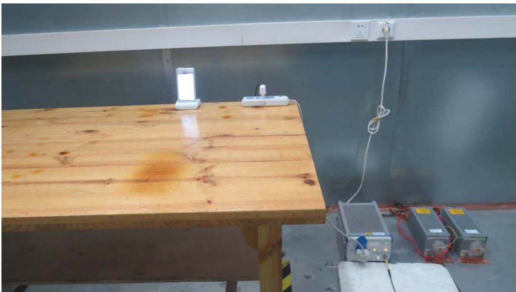
Picture 3 Conducted Emission Test Setup
