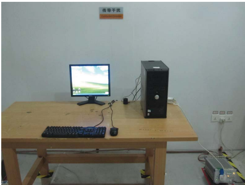
Photo of Setup for Conducted Emission Test
