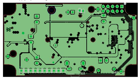
Power supply layer changes, part of the data line moved to the power supply layer, the IR lights go line also follow to do some adjustments
