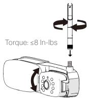
For the left/right side camera, ensure the lens on the camera is facing backwards and the MONITOR PAIRING button is facing downwards after installation.
