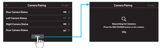
8. Press the **RED PAIRING** button at the bottom of the unpaired camera (left camera shown) to start the paring.
