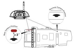
**NOTE:** The RV shown here is for reference only. You can mount Furrion Vision S+ products onto various types of RV such as trailers and Class A/B/C
