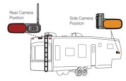
**NOTE:** The RV shown here is for reference only. You can mount Furrion Vision S+ products onto various types of RV such as trailers and Class A/B/C motorhomes.
