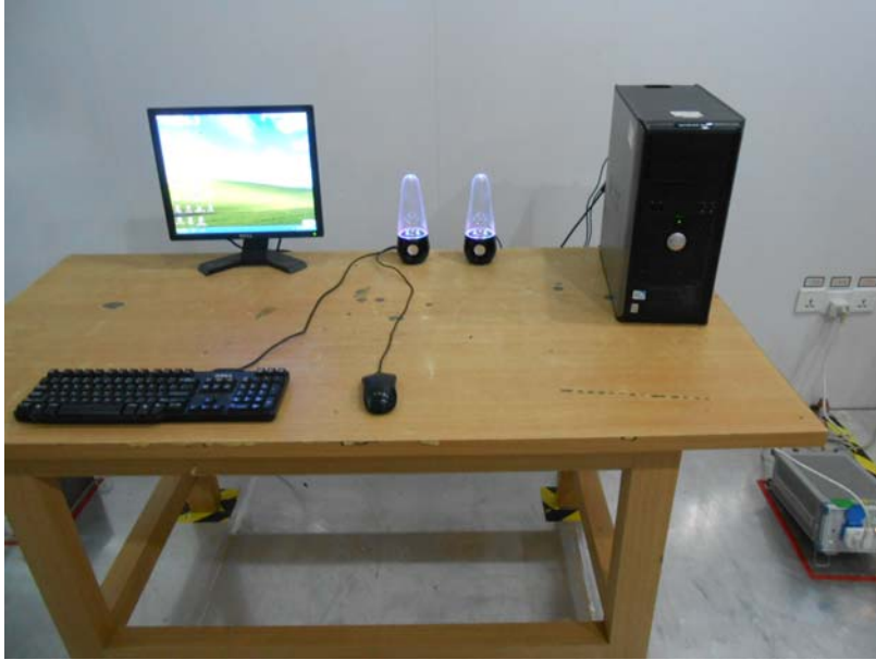
Photo of Setup for Conducted Emission Test
