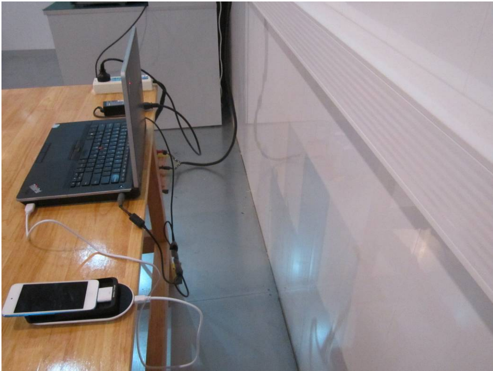
Conducted Emissions Test Setup Side View
