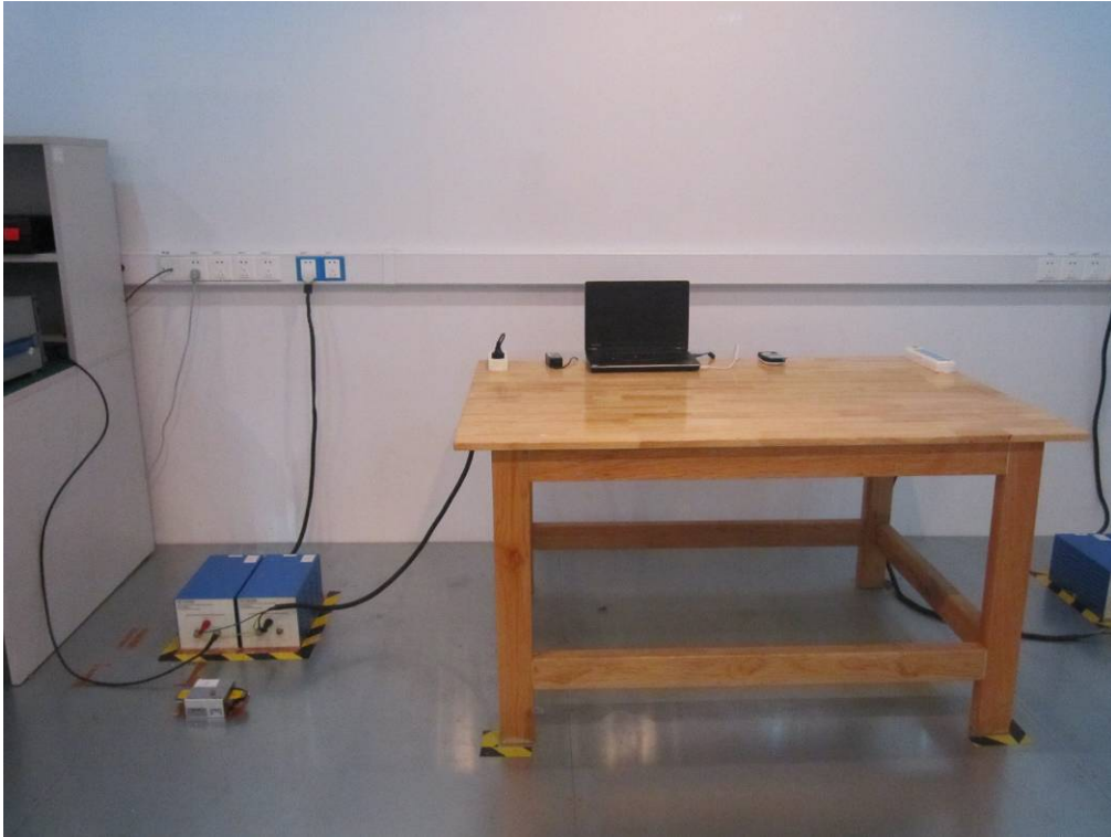
Conducted Emissions Test Setup Front View
