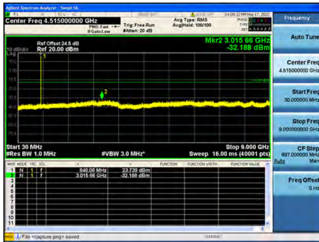
Band5 / 1.4MHz / High CH / 64QAM
