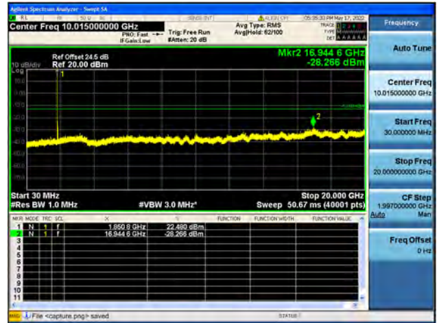
Band25 / 15MHz / Mid CH / QPSK
