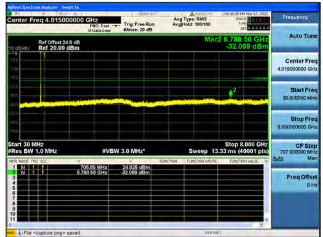
Band12 / 10MHz / High CH / 64QAM
