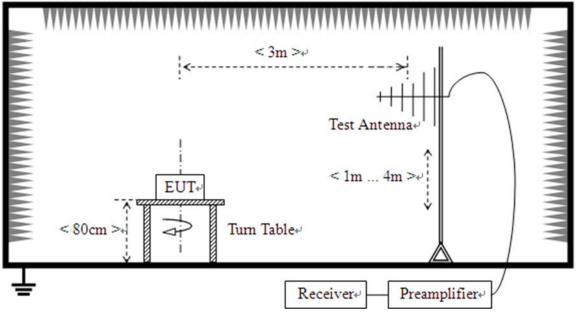
(For the test frequency from 30MHz to1GHz)
