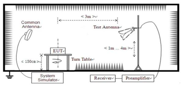
(For the test frequency above 1GHz)
