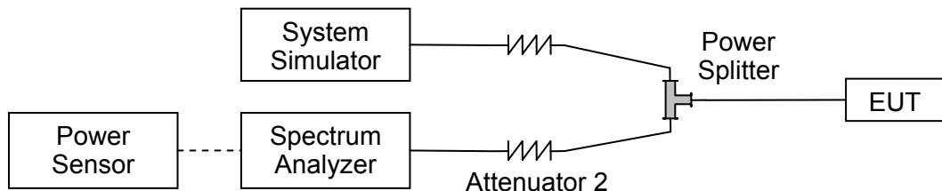
The EUT is coupled to the Spectrum Analyzer (SA) and the System Simulator (SS) with Attenuators through the Power Splitter; the RF load attached to the EUT antenna terminal is 50Ohm; the path loss as the factor is calibrated to correct the reading. The EUT is commanded by the SS to operate at the maximum output power i.e. Power Control Level (PCL) = 5 and Power Class = 4. A call is established between the EUT and the SS.
