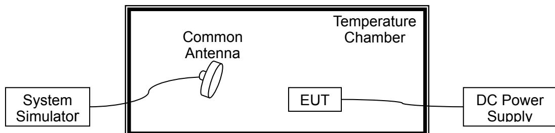
The EUT, which is powered by the DC Power Supply directly, is located in the Temperature Chamber. The EUT is commanded by the System Simulator (SS) to operate at the maximum output power i.e. Power Control Level (PCL) = 5 and Power Class = 4. A call is established between the EUT and the SS via a Common Antenna.
