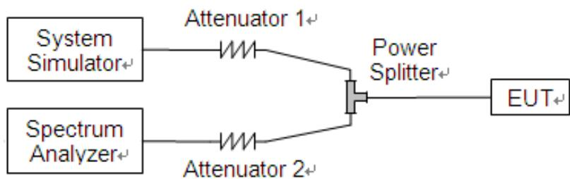
The EUT is coupled to the Spectrum Analyzer (SA) and the System Simulator (SS) with Attenuators through the Power Splitter; the RF load attached to the EUT antenna terminal is 50Ω; the path loss as the factor is calibrated to correct the reading. The EUT is commanded by the SS to operate at the maximum output power i.e. Power Control Level (PCL) = 5 and Power Class = 4. A call is established between the EUT and the SS.
