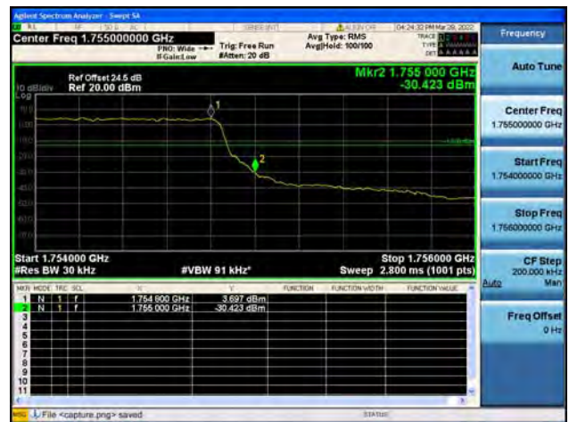
Band4 / 1.4MHz / High CH / QPSK / FULL RB
