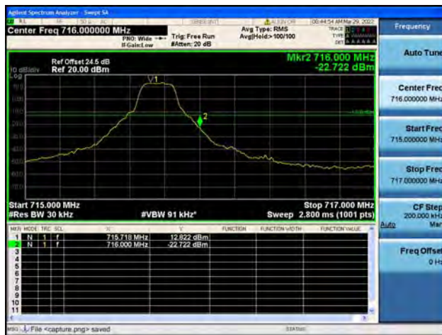
Band12 / 3MHz / High CH / QPSK / 1 RB
