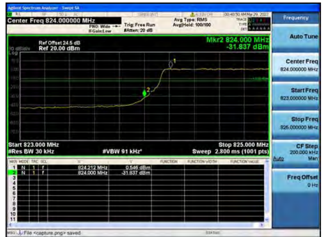
Band5 / 3MHz / High CH / QPSK / FULL RB
