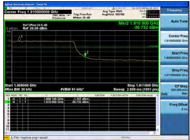
Band2 / 3MHz / High CH / QPSK / FULL RB
