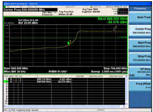
Band12 / 1.4MHz / High CH / QPSK / FULL RB
