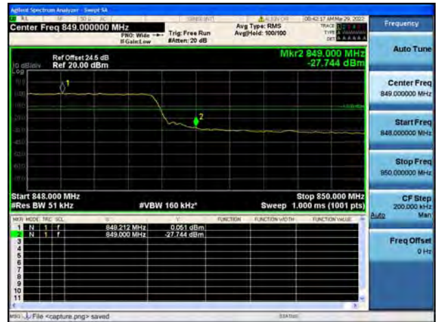
Band5 / 5MHz / High CH / QPSK / FULL RB
