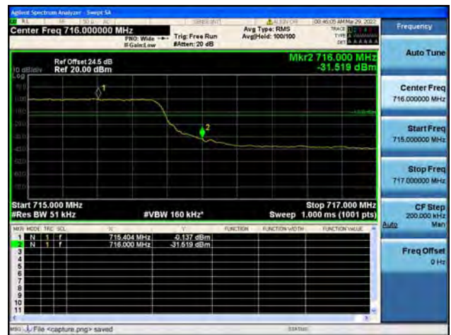
Band12 / 5MHz / High CH / QPSK / FULL RB
