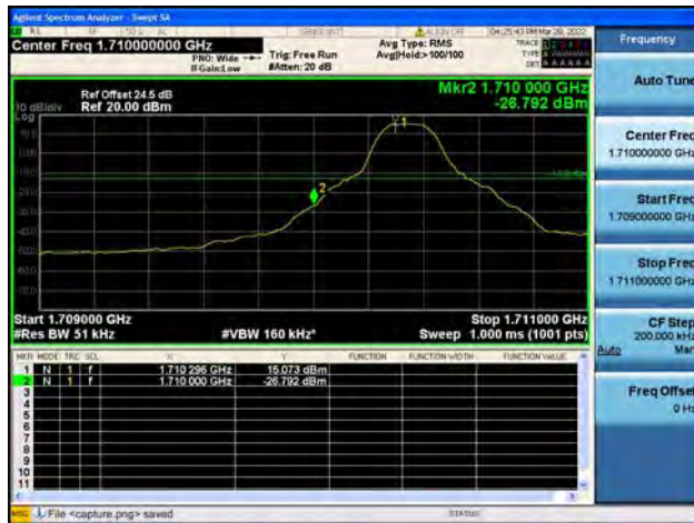
Band4 / 5MHz / High CH / QPSK / 1 RB
