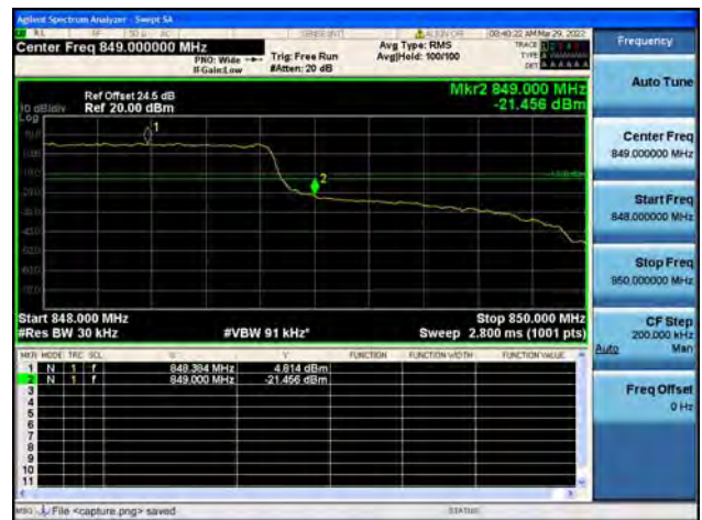
Band5 / 1.4MHz / High CH / QPSK / FULL RB
