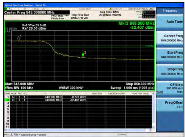
Band5 / 10MHz / High CH / QPSK / FULL RB
