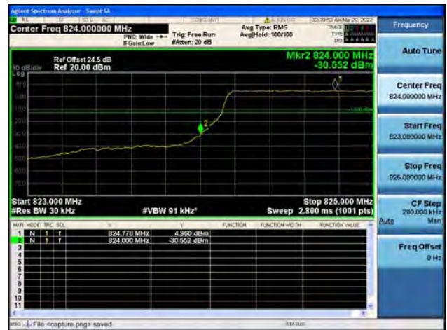
Band5 / 1.4MHz / High CH / QPSK / FULL RB
