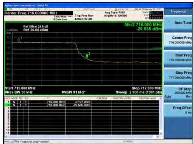
Band12 / 3MHz / High CH / QPSK / FULL RB
