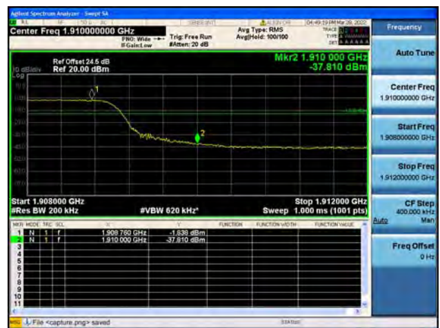
Band2 / 20MHz / High CH / QPSK / FULL RB
