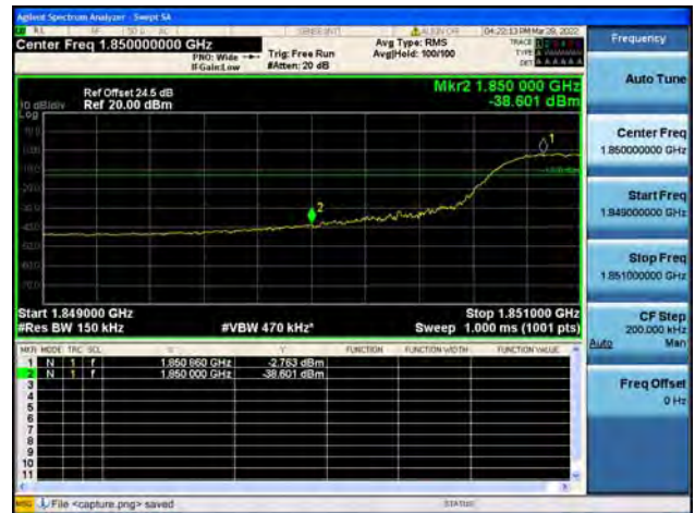
Band2 / 15MHz / High CH / QPSK / FULL RB
