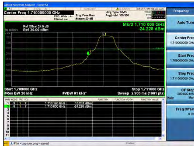
Band4 / 3MHz / High CH / QPSK / 1 RB
