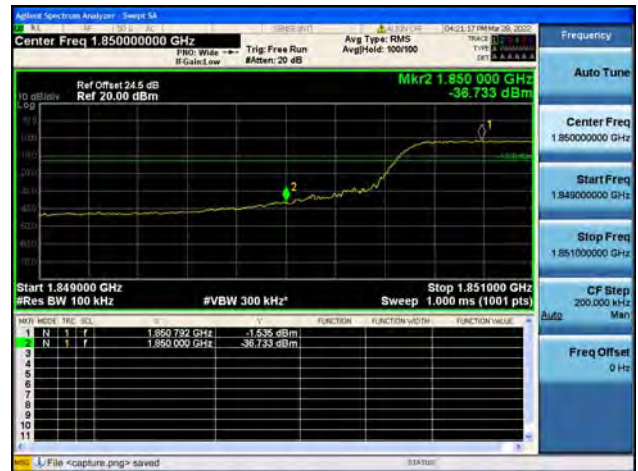
Band2 / 10MHz / High CH / QPSK / FULL RB
