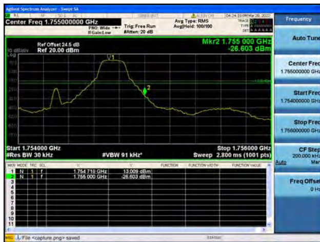
Band4 / 1.4MHz / High CH / QPSK / 1 RB
