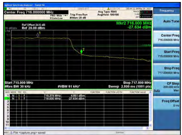
Band12 / 1.4MHz / High CH / QPSK / FULL RB
