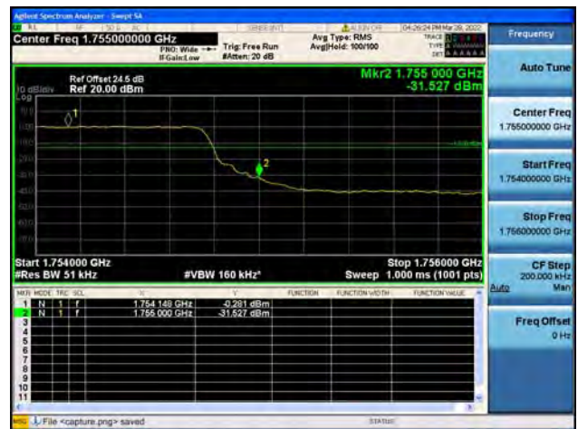
Band4 / 5MHz / High CH / QPSK / FULL RB
