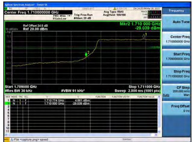
Band4 / 1.4MHz / High CH / QPSK / FULL RB
