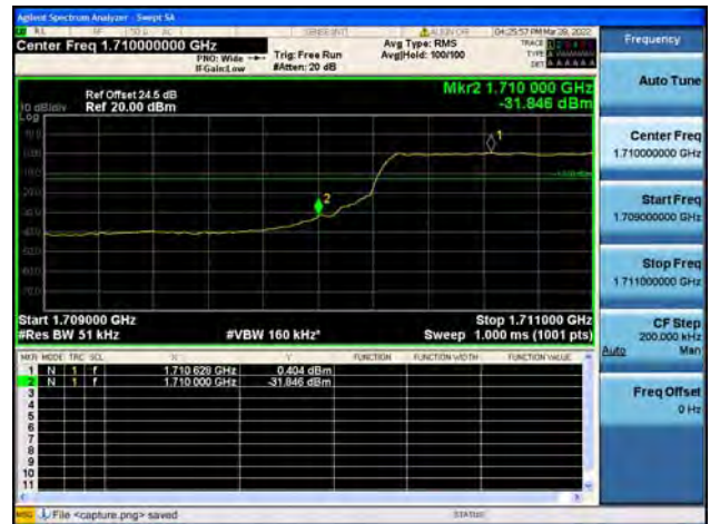
Band4 / 5MHz / High CH / QPSK / FULL RB
