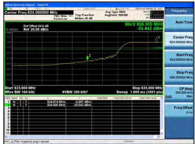
Band5 / 10MHz / High CH / QPSK / FULL RB
