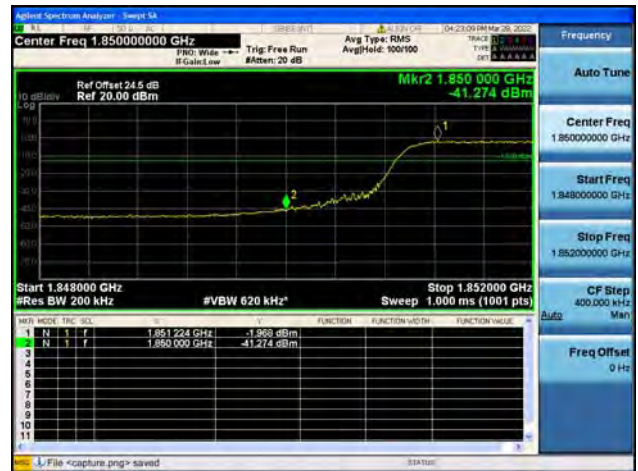
Band2 / 20MHz / High CH / QPSK / FULL RB
