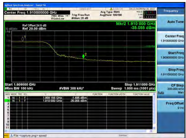
Band2 / 10MHz / High CH / QPSK / FULL RB
