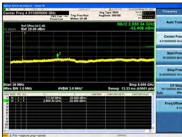
Band17 / 5MHz / High CH / QPSK
