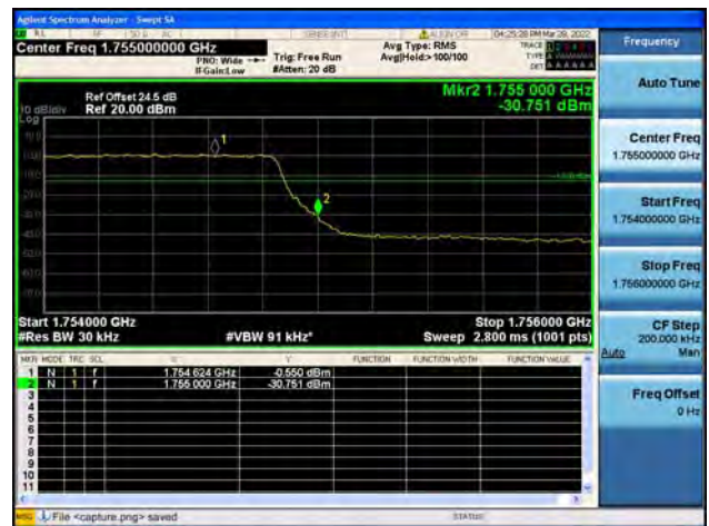
Band4 / 3MHz / High CH / QPSK / FULL RB
