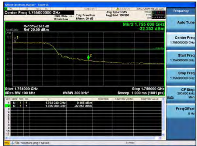
Band4 / 10MHz / High CH / QPSK / FULL RB
