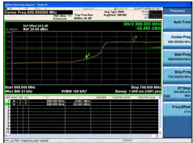
Band12 / 5MHz / High CH / QPSK / FULL RB
