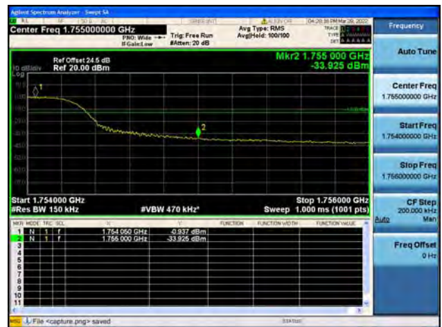
Band4 / 15MHz / High CH / QPSK / FULL RB
