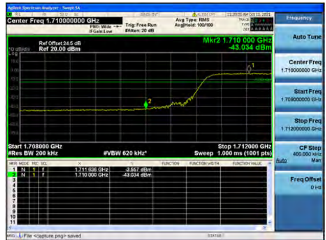
Band4 / 20MHz / High CH / QPSK / FULL RB
