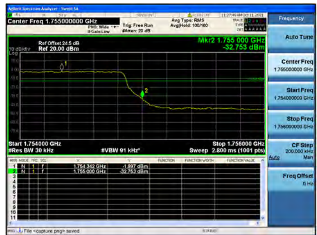
Band4 / 3MHz / High CH / QPSK / FULL RB
