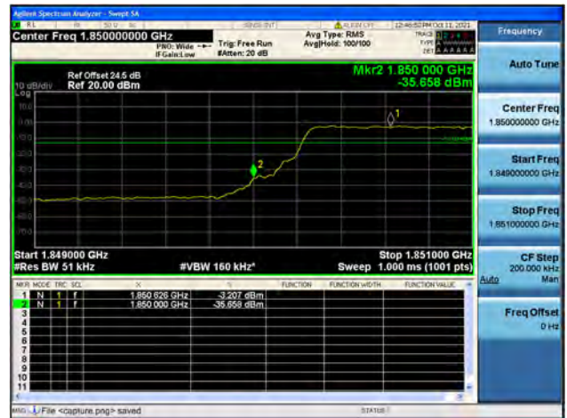
Band25 / 5MHz / High CH / QPSK / FULL RB
