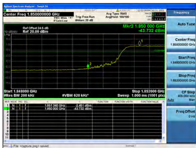
Band25 / 20MHz / High CH / QPSK / FULL RB
