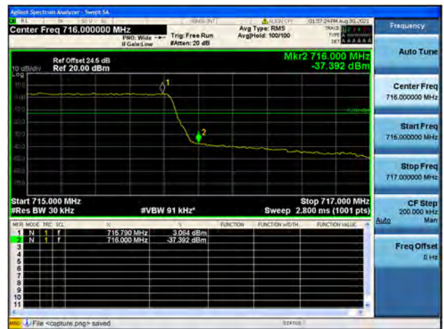
Band12 / 1.4MHz / High CH / QPSK / FULL RB
