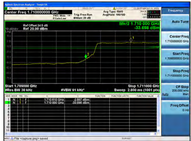
Band4 / 3MHz / High CH / QPSK / FULL RB
