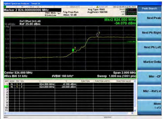
Band26 / 5MHz / High CH / QPSK / FULL RB
