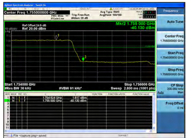
Band4 / 1.4MHz / High CH / QPSK / FULL RB
