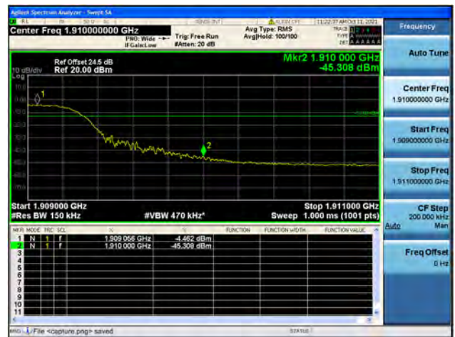
Band2 / 15MHz / High CH / QPSK / FULL RB
