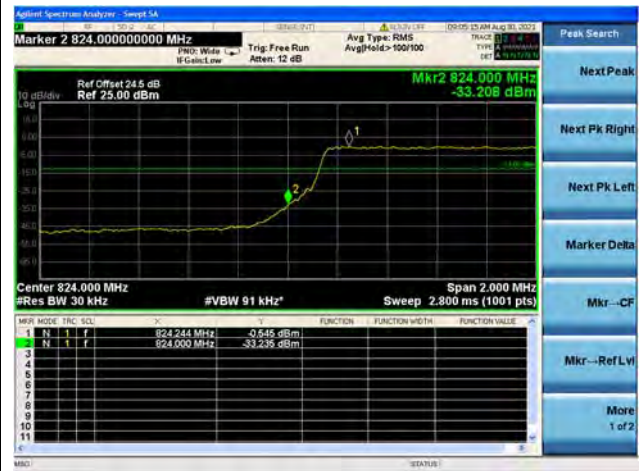
Band26 / 3MHz / High CH / QPSK / FULL RB
