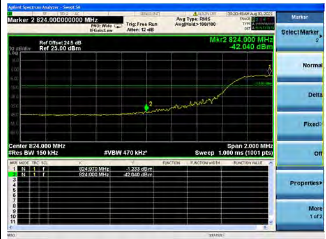
Band26 / 15MHz / High CH / QPSK / FULL RB
