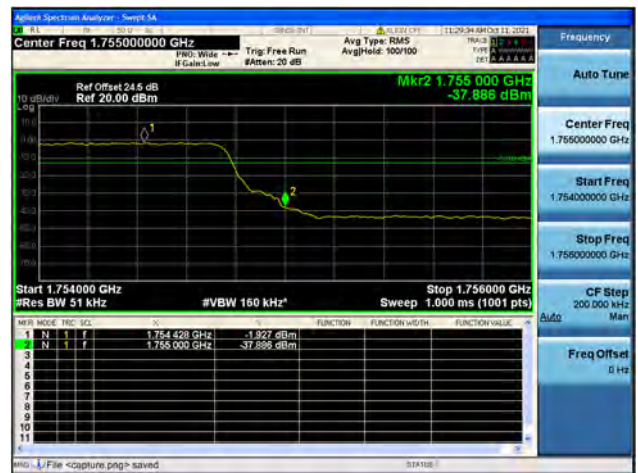
Band4 / 5MHz / High CH / QPSK / FULL RB
