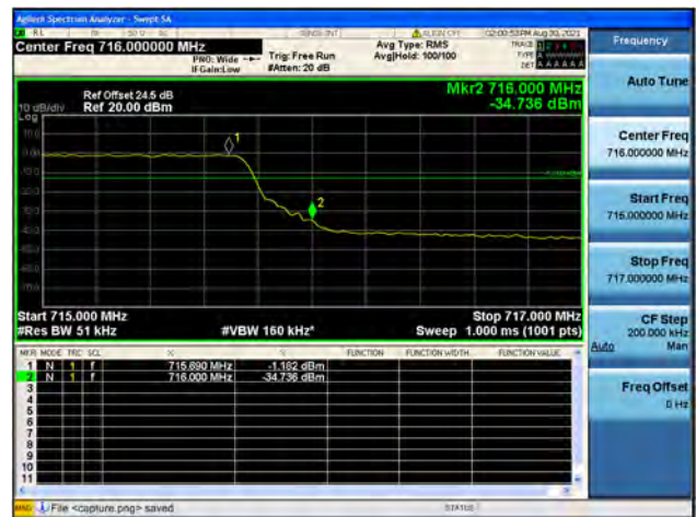
Band12 / 5MHz / High CH / QPSK / FULL RB
