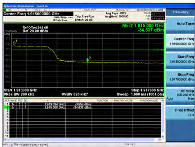
Band25 / 20MHz / High CH / QPSK / FULL RB
