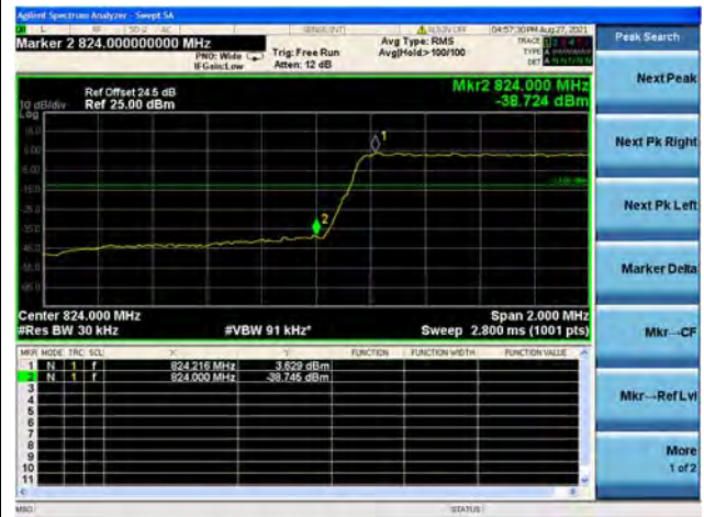
Band26 / 1.4MHz / High CH / QPSK / FULL RB
