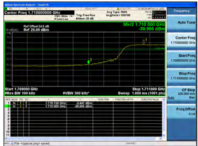
Band4 / 10MHz / High CH / QPSK / FULL RB
