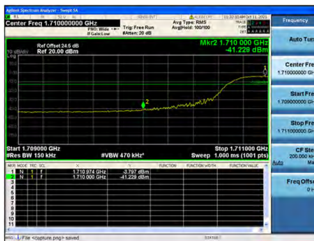
Band4 / 15MHz / High CH / QPSK / FULL RB
