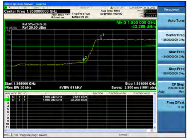
Band25 / 1.4MHz / High CH / QPSK / FULL RB
