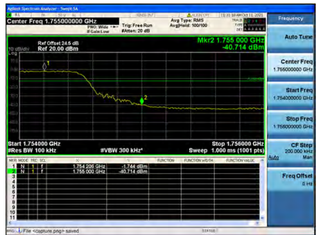
Band4 / 10MHz / High CH / QPSK / FULL RB
