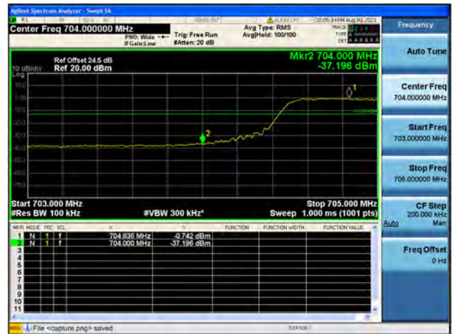
Band17 / 10MHz / High CH / QPSK / FULL RB
