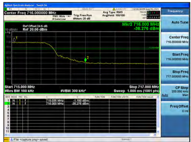
Band17 / 10MHz / High CH / QPSK / FULL RB
