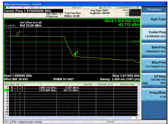
Band2 / 1.4MHz / High CH / QPSK / FULL RB
