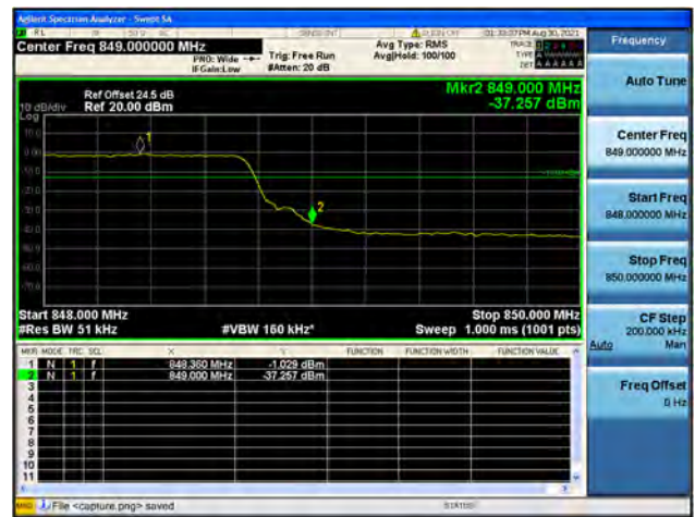
Band5 / 5MHz / High CH / QPSK / FULL RB
