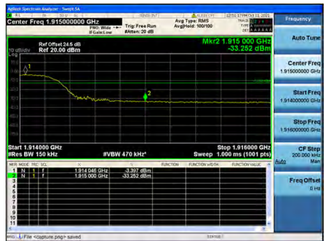
Band25 / 15MHz / High CH / QPSK / FULL RB
