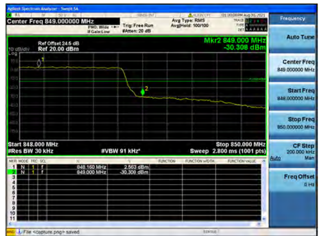
Band5 / 1.4MHz / High CH / QPSK / FULL RB
