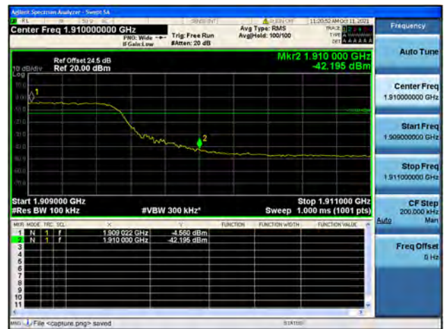
Band2 / 10MHz / High CH / QPSK / FULL RB
