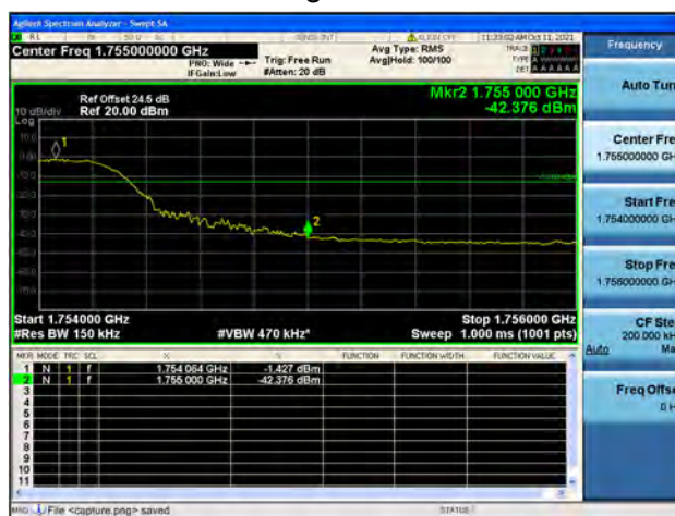
Band4 / 15MHz / High CH / QPSK / FULL RB
