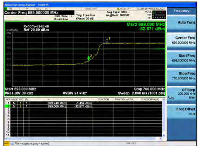
Band12 / 3MHz / High CH / QPSK / FULL RB
