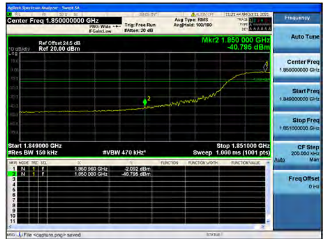
Band2 / 15MHz / High CH / QPSK / FULL RB
