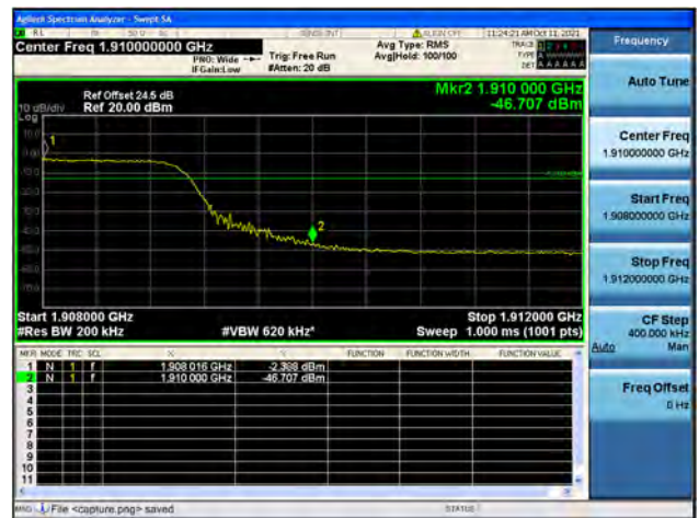
Band2 / 20MHz / High CH / QPSK / FULL RB
