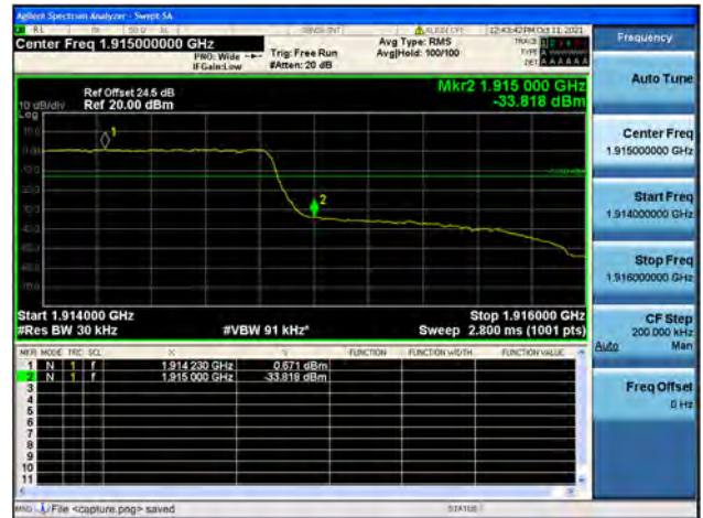
Band25 / 1.4MHz / High CH / QPSK / FULL RB
