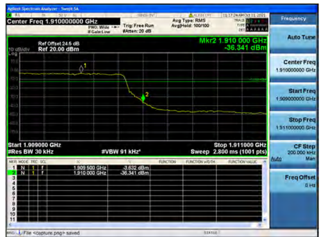
Band2 / 3MHz / High CH / QPSK / FULL RB
