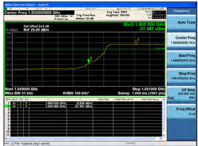
Band2 / 5MHz / High CH / QPSK / FULL RB
