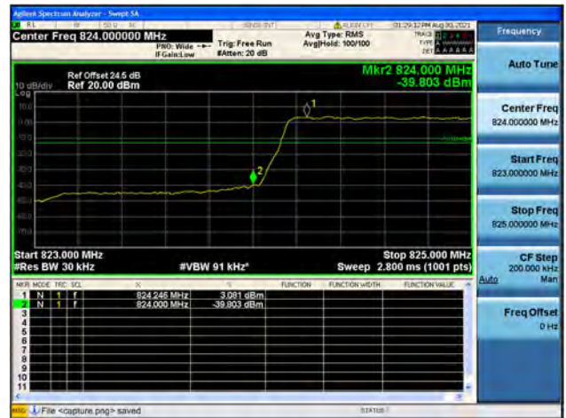
Band5 / 1.4MHz / High CH / QPSK / FULL RB
