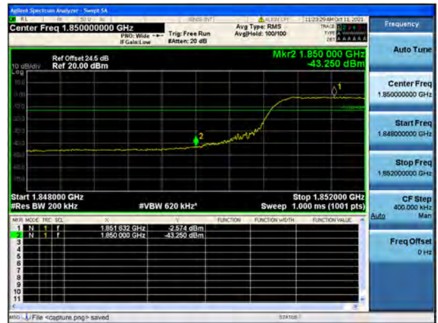
Band2 / 20MHz / High CH / QPSK / FULL RB
