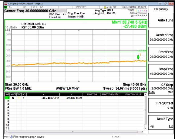
5A\_n77(3700-3980MHz) (20GHz-40GHz) 60M DFT-s-OFDM BPSK Outer\_Full High
