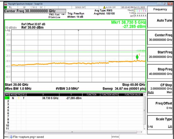
5A\_n77(3700-3980MHz) (20GHz-40GHz) 70M DFT-s-OFDM BPSK Edge\_1RB\_Left Low
