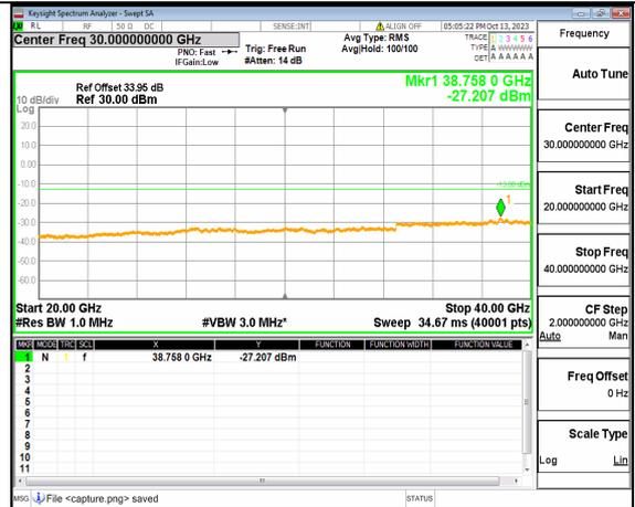
5A\_n77(3700-3980MHz) (20GHz-40GHz) 60M DFT-s-OFDM QPSK Outer\_Full High
