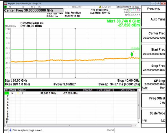
5A\_n77(3700-3980MHz) (20GHz-40GHz) 40M DFT-s-OFDM QPSK Outer\_Full Mid
