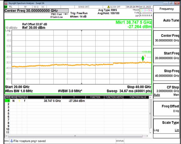
5A\_n77(3700-3980MHz) (20GHz-40GHz) 50M DFT-s-OFDM QPSK Outer\_Full Low
