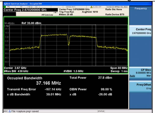
Band41C / 20MHz+20MHz / 64QAM/ High CH
