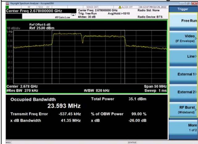
Band41C / 10MHz+15MHz / 64QAM/ High CH
