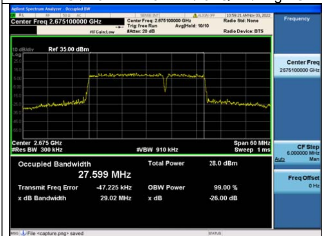
Band41C / 20MHz+10MHz / 16QAM/ High CH
