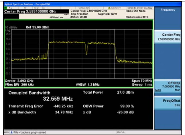
Band41C / 20MHz+15MHz / 16QAM/ Mid CH
