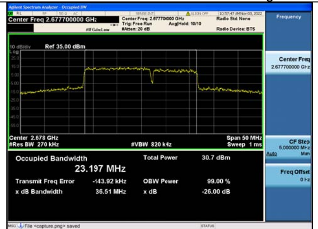
Band41C / 15MHz+10MHz / QPSK/ High CH
