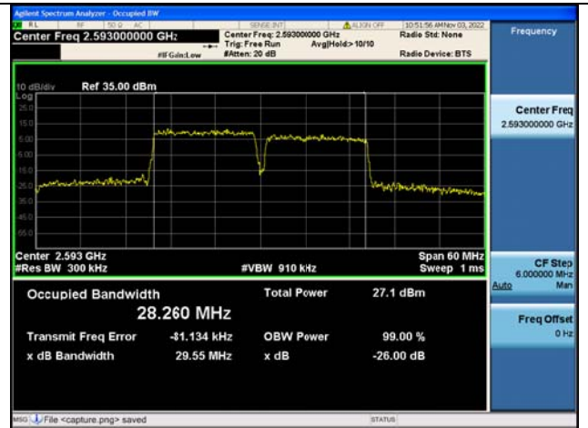
Band41C / 15MHz+15MHz / 16QAM/ Mid CH
