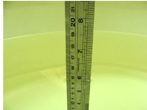
Fig 7.2 Photo of Liquid Height for Body SAR
