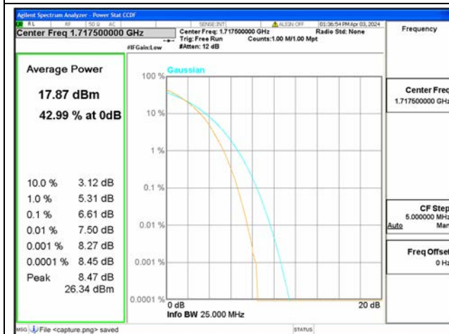
B4 / 15MHz / Low CH / 64QAM
