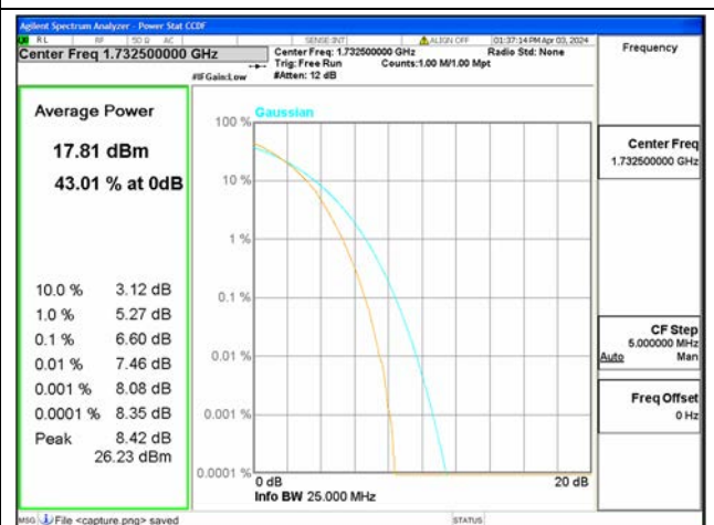
B4 / 15MHz / Mid CH / 64QAM
